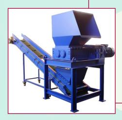
The segments of the shredder are made of highquality steel. The shear clearance betwoon the opposite segments is about some tenths of millimetres.
